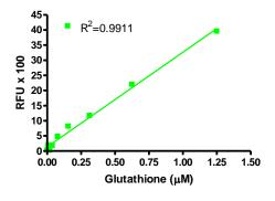
Figure 2. Expanded lower concentration range using the SensoLyte® 520 Thiol Quantitition Kit. Fluorescence signal was detected at Ex/Em=490/520 nm (FlexStation 384II).
