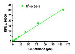
Figure 1. Detection of GSH with SensoLyte® 520 Quantitation Kit. Fluorescence signal was detected at Ex/Em=490/520 nm (FlexStation 384II).
