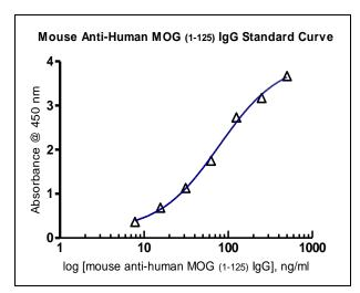
$Y=[(A-D)/(1+\{x/C\}^AB)]+D, \underline{A}=0.1647 \underline{B}=1.206 \underline{C}=78.15 \underline{D}=4.013 R^2=0.997$
